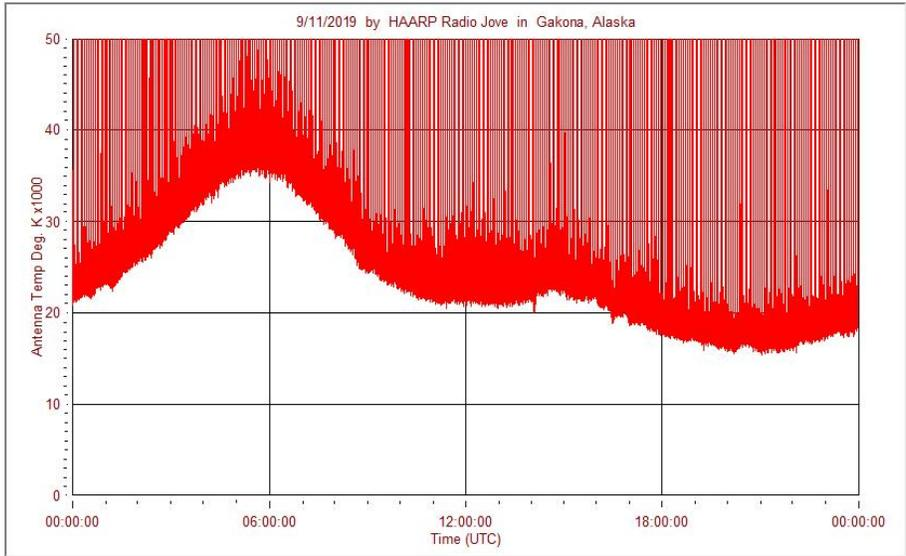
Figure 4.d ~ Averaging bin size = 10x10x10x10. Note the baseline rise is not as high as the ordinary smoothing used in figure 3.
