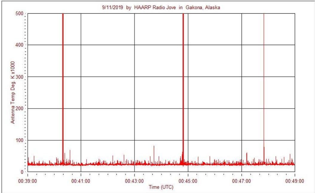
Figure 1 ~ 10 min plot of Radio-SkyPipe data from 11 September 2019 as received by the Radio JOVE receiver and dual dipole antenna at HAARP. Three strong pulses are visible in the plot at 0040:20, 0044:50 and 0047:50. This pattern repeats 24 h d<sup>-1</sup>. The noise baseline represents the galactic background radiation at 20.1 MHz.
