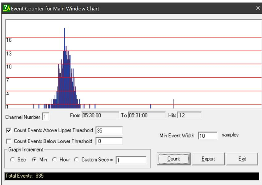
Figure 7 ~ The *Event Counter* is setup to show the number of events that exceed 35 000 K in a 1 min interval with a minimum width of 1 s (10 samples at 100 ms s<sup>-1</sup>). For this screenshot the mouse cursor was placed at the location of the peak count corresponding to the 0530 to 0531 interval. Although this plot may give the impression that the peak is sharp, in reality it is quite broad.
