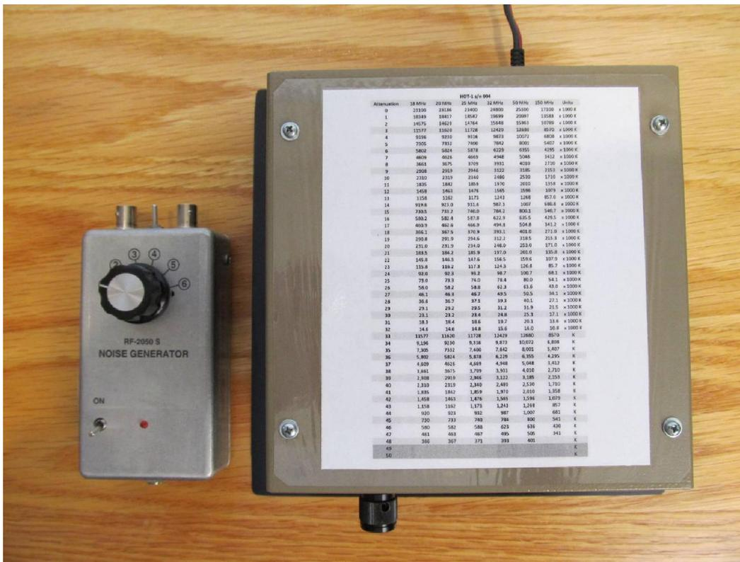
Figure 6 ~ Packaged HOT-1 with calibration chart (right) next to RF-2050S (left). The calibration chart was laminated and fastened to the top of the enclosure with small self-threading screws and washers.
