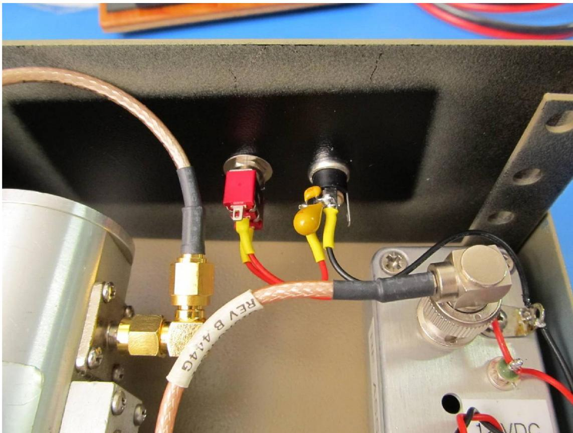
Figure 4 ~ Close-up of the filter capacitors soldered directly to the coaxial dc power jack on the rear panel. The panel was factory painted black, and some overspray from the new color, dark taupe, can be seen around the components.
