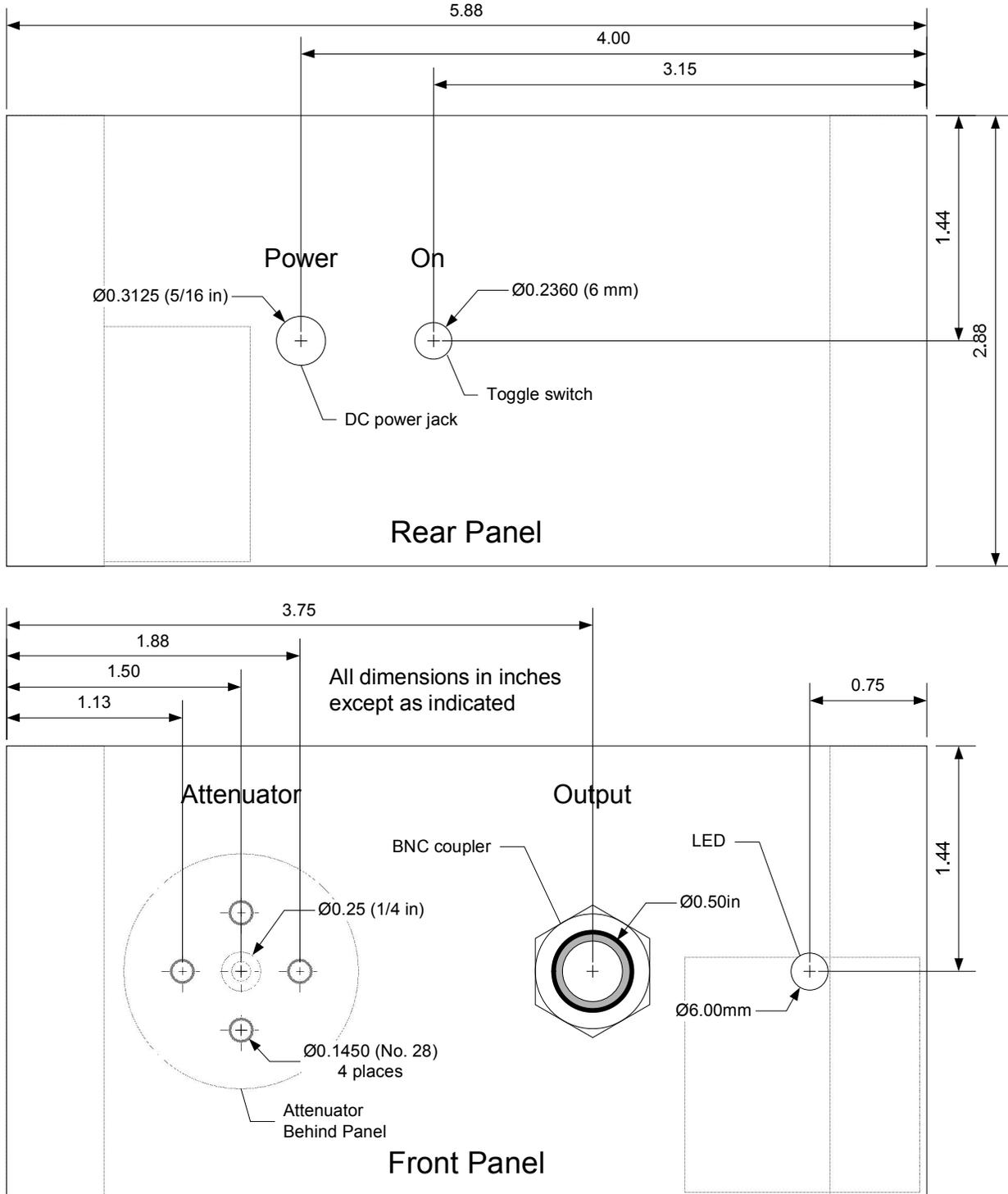
Figure 2 ~ Front and rear panel layouts for the HOT-1 Package. Dimensions shown correspond to the items listed in the bill of materials.
