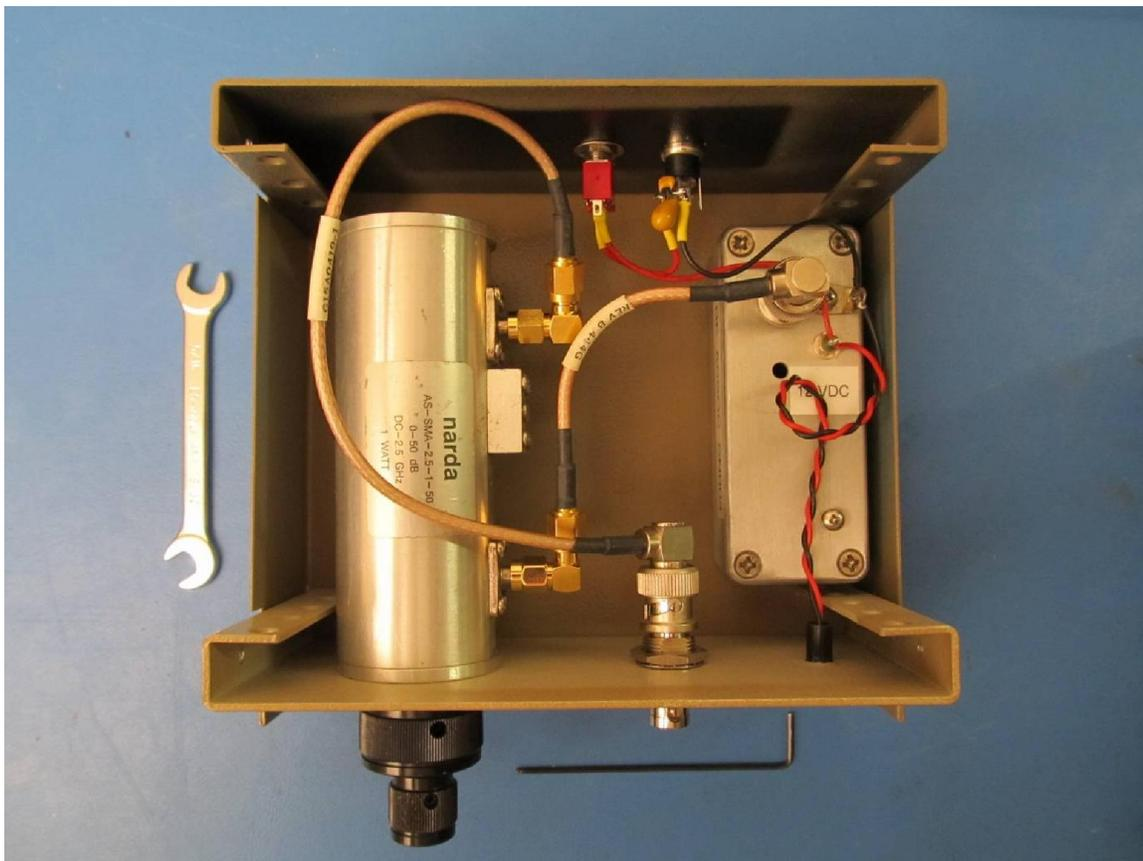
Figure 1 ~ Top view of the painted metal enclosure, which includes an RF Associates HOT-1 noise generator (right) and attenuator (left). The enclosure also includes a power switch and power input jack (top) and a BNC connector for the output (bottom). The 5/16 in wrench is for the SMA connectors and a 1/16 in hex L-wrench is for the attenuator knobs.
