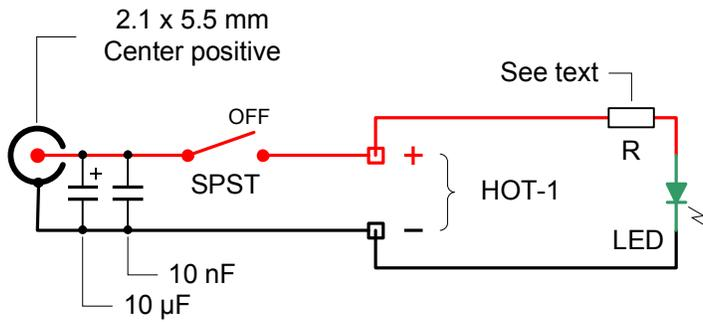
Figure 3 ~ Power wiring schematic. The current limiting resistor, R, is not required if the specified LED is used.
