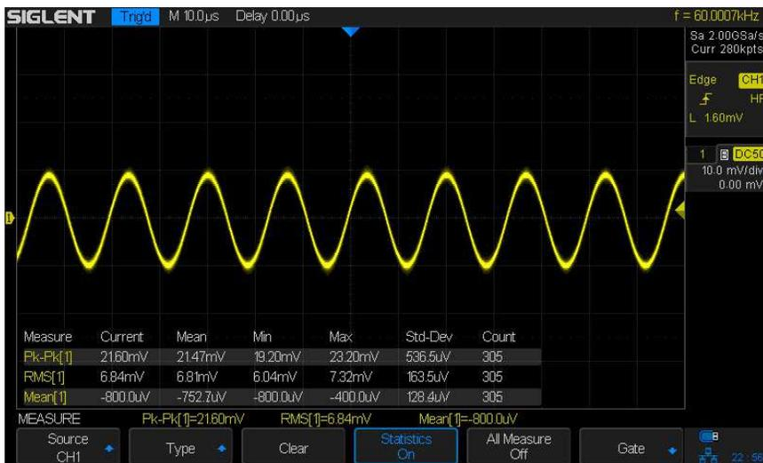
Figure A.3 ~ U402 Replaced L3, L4. Image © 2019 W. Reeve
