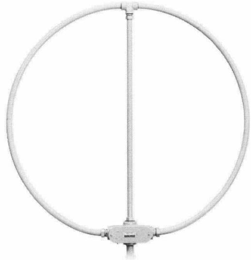
The loop antenna is made from heavy-duty aluminum tubing and includes a built-in double-tuned preamplifier assembly mounted inside a cast aluminum enclosure at the base of the antenna. The only external connection is through a BNC-F connector for a coaxial cable that carries dc power to and RF signal from the preamplifier. The original system was designed for up to 1000 ft (300 m) of cable.
