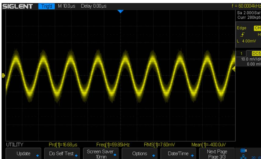
Figure 17.a ~ New dual J-FET preamplifier test output. The measured voltage is 7.60 Vrms for an arbitrary 60 kHz input to the coupling loop. For these measurements the oscilloscope vertical amplifier was set for X1 probe and to terminate the coaxial input with 50 ohms. Image © 2019 W. Reeve
