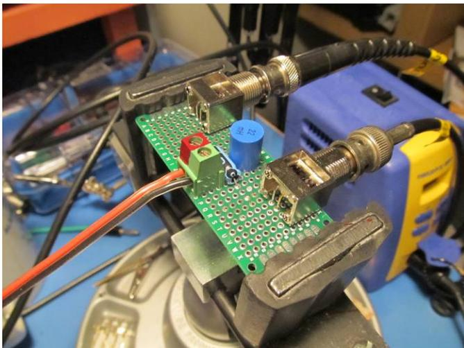
Lower: Circuit built on prototype PCB material and mounted in a PanaVise during use.
