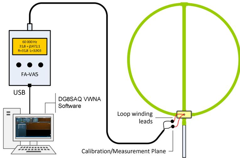
Figure 12 ~ Measurement setup using the FA-VA5 Vector Antenna Analyzer and DG8SAQ VNWA software. The analyzer was calibrated with the same coaxial cable used in the measurements. The calibration and measurement planes were at the end of the coaxial cable clip leads. The analyzer was controlled by the VNWA software rather than the keyboard due to limitations with its pushbutton controls. Image © 2019 W. Reeve
