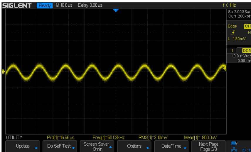
Figure 16.b ~ Original Nuvistor preamplifier output. The measured voltage is 3.10 Vrms for the same conditions as above. Image © 2019 W. Reeve
