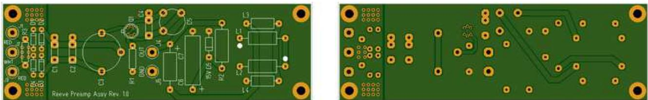
Figure 4 ~ Preamplifier 2-layer printed circuit board showing (left) top/component side and (right) bottom side (reversed from actual). The thin separation of the two reference grounds is visible near the left side of the images. The loop connects to the three terminals on the far-left between the mounting holes. The power input/RF output terminals are near the middle of the PCB. Images are rendered by a viewer that uses the PCB Gerber files.
