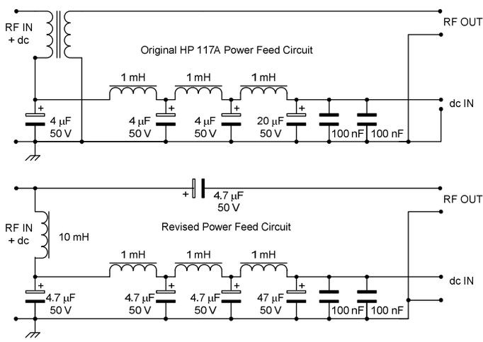
Figure 9 ~ Upper schematic: Original HP power feed circuit. The HP circuit isolates the receiver from the power supply with an input coupling transformer. The HP transformer was specially made and no longer available. The corner (3 dB) frequency of the pi-filter is 3 kHz and it introduces 40 dB attenuation at 6 kHz as determined with the AADE Filter Design software tool.
