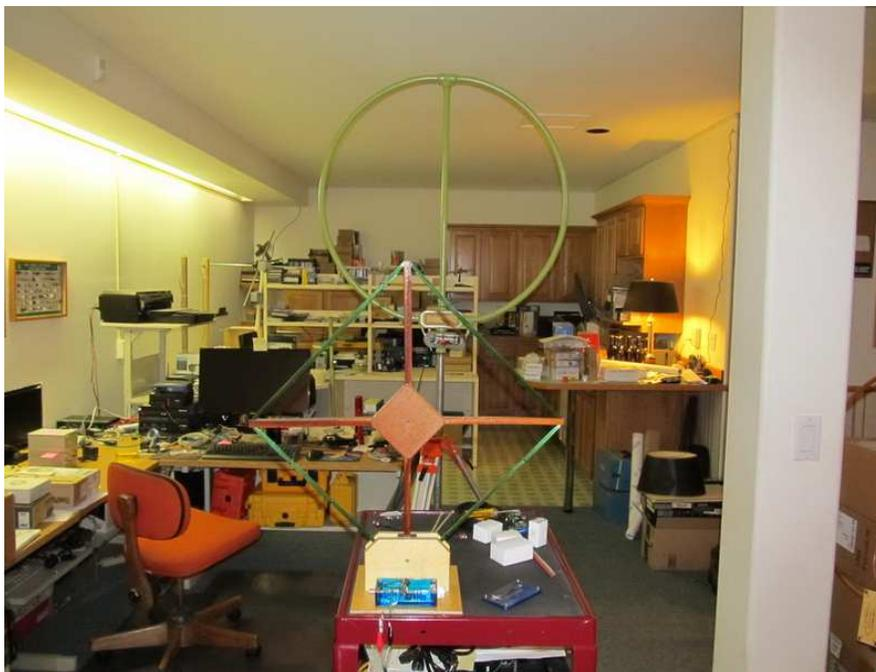
Figure 14 ~ Measurement setup with square signal loop wound with green coated wire in the foreground. Separation between the two loops was a couple meters and not critical. Note that the flat sides of the loops are approximately parallel. The separation and orientation were held constant for all comparative measurements. Image © 2019 W. Reeve
