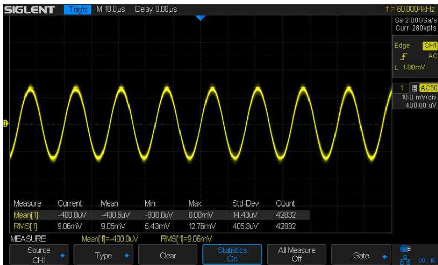
Figure A.4 ~ U402 Replaced R1 with trimmer resistor and adjusted bias to 0.6 V. Image © 2019 W. Reeve
