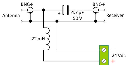
Figure 8 ~ Upper: Schematic of a simple bias-tee circuit used for initial preamplifier testing. It consists of a single inductor and electrolytic capacitor for the lowpass filter, two BNC-F connectors for the RF connections and a terminal block for the dc power connection. The reactance of the inductor at 60 kHz is about 8300 ohms and provides plenty of dc power supply isolation. The reactance of the capacitor is about 0.6 ohms and essentially is a short-circuit to the RF.
