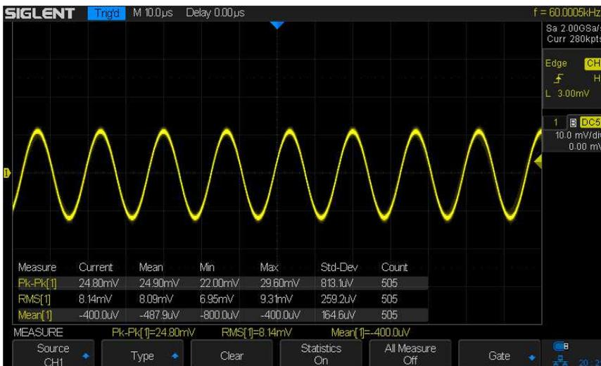
Figure A.1 ~ U402-2 Baseline. In this and following images, a statistics table shows mean, minimum, maximum, standard deviation, and average count for peak-peak voltage, rms voltage and average voltage. Image © 2019 W. Reeve
