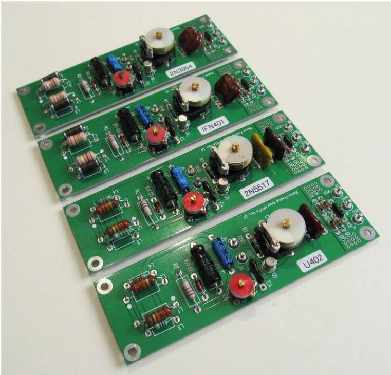
Figure 6 ~ Four of five new preamplifiers used for testing and measurements. The output transformer composed of four fixed inductors is on the far-left of each board and the antenna turret terminals are on the far-right. The red trimmer capacitor near the middle-edge of the PCB tunes the output and the white trimmer capacitor to the right tunes the input. Each PCB is labeled with the dual J-FET transistor type. Image © 2019 W. Reeve
