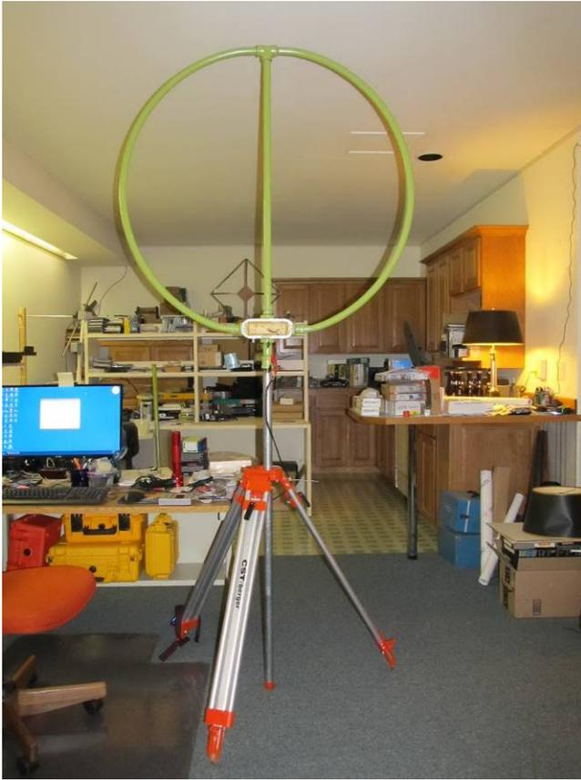
Figure 11 ~ Loop antenna on tripod test stand in the lab. The loop is supported by a 4 ft (1.2 m) length of 1 in (25 mm) galvanized steel pipe that is attached to the tripod. This setup was used for all measurements. Image © 2019 W. Reeve
