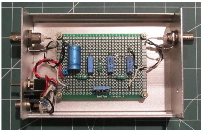
Figure 10 ~ Upper: Prototype PCB for power feed circuit in an enclosure and wired for service. The extruded aluminum enclosure is 110 x 80 x 36 mm. The end panels include a power switch, power input jack and associated protective and noise filter circuitry, power indicating LED, and BNC-F connectors for RF input + dc and RF output.
