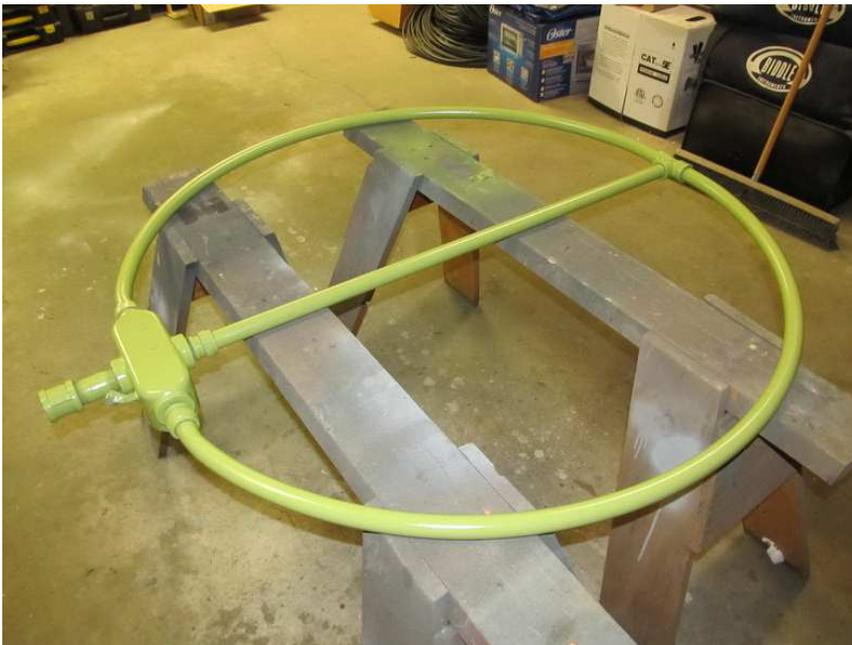
Figure 2 ~ Loop antenna sitting on saw horses after the paint has cured for 48 h. The threaded pipe coupling for mast mounting can be seen on the left, where it is connected to the preamplifier housing. Image © 2019 W. Reeve
