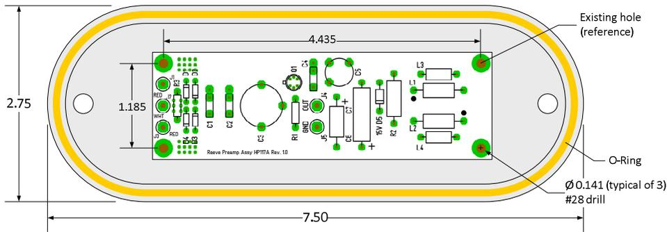
Figure 7 ~ Antenna base enclosure cover dimensional drawing. The cover has three holes for the original vacuum tube preamplifier but only one of them is used with the new preamplifier. Image © 2019 W. Reeve
