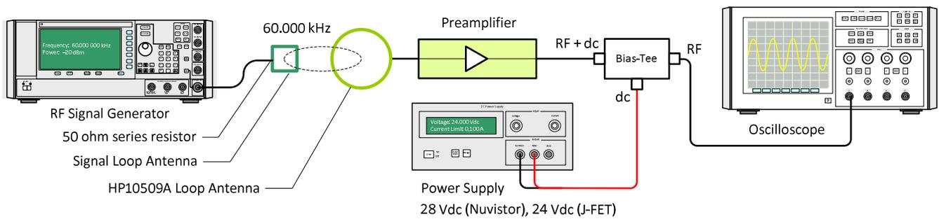
Figure 15 ~ Test setup for the preamplifiers includes the smaller test signal loop for coupling the 60 kHz test signal from a signal generator. The test signal flows left-to-right. The preamplifier output was measured with an oscilloscope setup with 50 ohms termination and X1 probe setting. Image © 2019 W. Reeve
