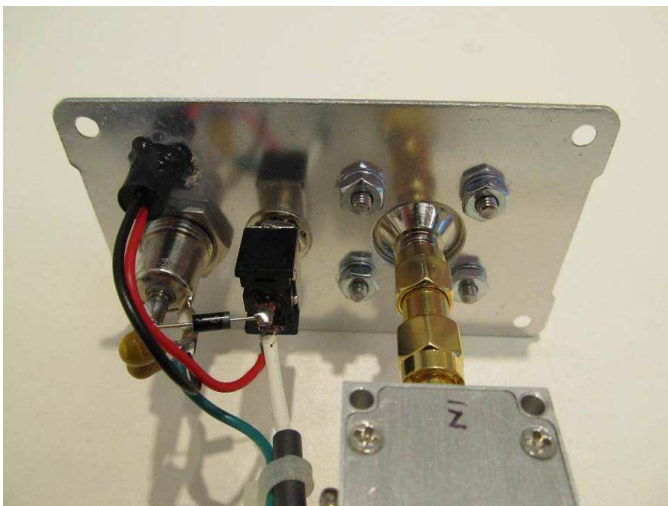
Figure 5 ~ Close-up of the inside front panel showing the input filter capacitors soldered directly to the coaxial dc power jack on the left, polarity-guard diode and switch. The filter inductor from the power switch to the amplifier module is in lower-center and secured with a cable tie to the amplifier ground lead.
