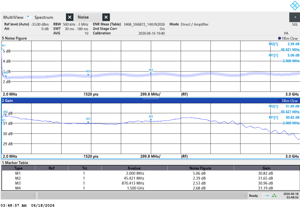
Figure 11.b ~ HP 8447A Modified (15 dB ENR)
