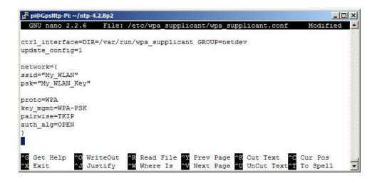
If you have more than one Wi-Fi network, you can add each of them to the wpa\_supplicant.conf file. The RPi will then connect to the one with the best signal. For a setup with multiple networks, the text lines "network = { additional network details }" will need to be determined and specified for each network.
