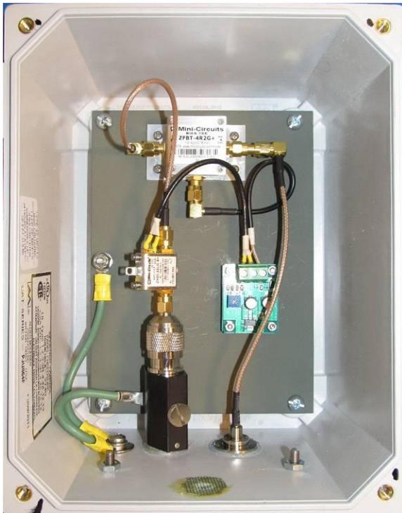
Figure 4 ~ Tower-mounted low noise amplifier. The TMA shown is a prototype, which used an adjustable internal voltage regulator (middle-right). The bias-tee is at top and the LNA module is middle-left. The black object at bottom-left is a lightning arrester.
