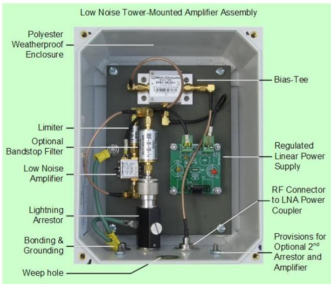
Figure 9 ~ Physical installation of the VLM-33+ voltage limiter in the TMA. It is connected directly to the LNA module RF output port shown left of middle. The TMA shown here is a production model that is equipped with a fixed low-voltage dropout linear regulator and an optional FM broadcast bandstop filter.
