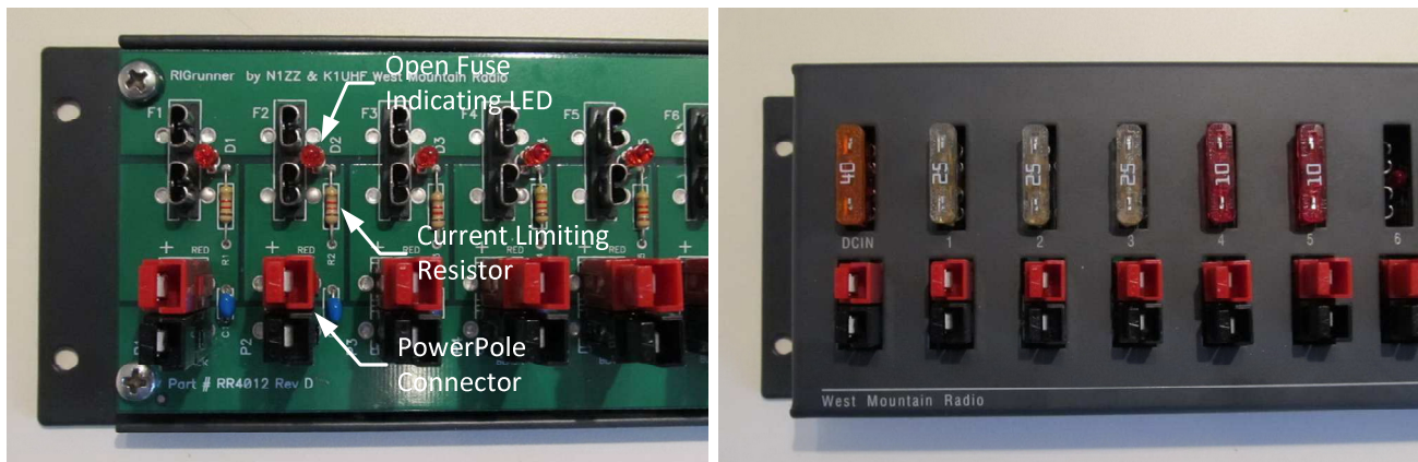
Figure 1. Left : Cover removed from a RigRunner distribution panel. The blown-fuse indicator LEDs on the printed circuit board can be seen just to the right of and between the two fuse blade sockets. The 1200 ohm current limiting resistors are
