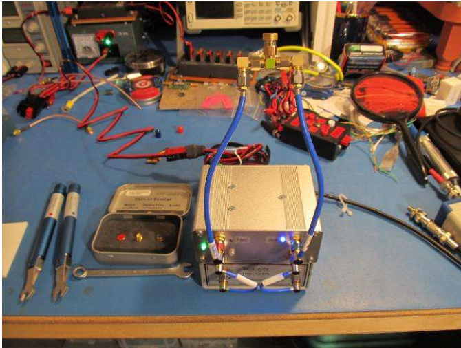
Figure 10 ~ T-Check connections. A coaxial tee-junction (top-center of image at end of blue cables) with 50 ohm load on the branch is inserted between the two test set ports after calibration (calibration includes the two test cables). The resulting s-parameter measurements are then used in the T-Check formula to calculate deviation from the ideal parallel 25 ohm impedance (50 ohm load in parallel with 50 ohm receive port on the VNWA-3E). Image © 2016 W. Reeve
