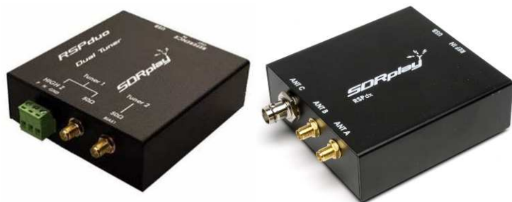
Figure 1 ~ The RSPduo (left) and RSPdx (right) SDR receivers cover the same frequency range – 1 kHz to 2 GHz. The RSPduo has two internal tuners and the RSPdx is a redesigned RSP2Pro with additional low frequency filters. The RSPdx is slightly larger at 4.4 L x 3.7 W x 1.4 H in (113 x 94 x 35 mm). Both receivers have a connector on the back panel for an external reference frequency source. Not shown are the RSP2 and RSP2Pro. Images source: SDRPlay
