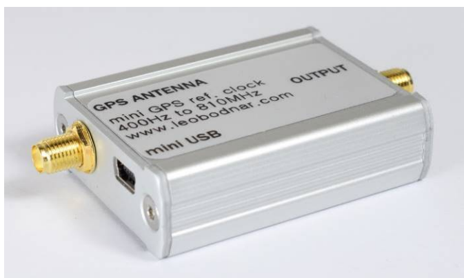
Figure 3 ~ Leo Bodnar Mini-GPS Reference Clock shown approximately full size. Dimensions are 2.1 L x 1.6 W x 0.7 H in (53 x 40 x 17 mm). The GPS antenna is connected through the SMA-F connector on the left; the output is on the other end and also uses an SMA-F connector. A mini-USB connector next to the GPS antenna connector is used for power from a 5 Vdc source. The unit may be connected to a PC USB port to set the frequency and output level and check satellite status. Image source: www.leobodnar.com
