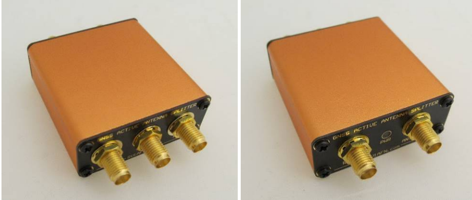
Figure 12 ~ SV1AFN GNSS 4-port antenna splitter. One receiver port is used to supply dc power to the antenna port (right). The other three ports (left) provide a passive load to the receiver antenna inputs to prevent an “antenna fail” alarm condition. Dimensions are 1.9 L x 1.7 W x 0.7 in H (49 x 44 x 18 mm). Images © 2020 W. Reeve
