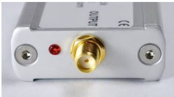
Figure 4 ~ Mini-GPS Reference Clock front panel showing the output connector and unlabeled status LED to the left of the connector. Image source: www.leobodnar.com
