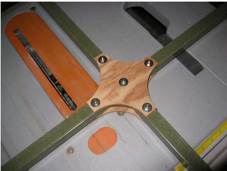
After sanding the reinforcements, they were clamped to the braces to ensure alignment and drilled with a 3/16 in brad point drill. The fasteners are 18-8 stainless steel 10-32 machine screws, washers and nuts. After this image was taken, the wood pieces were removed and painted with urethane spar varnish.
