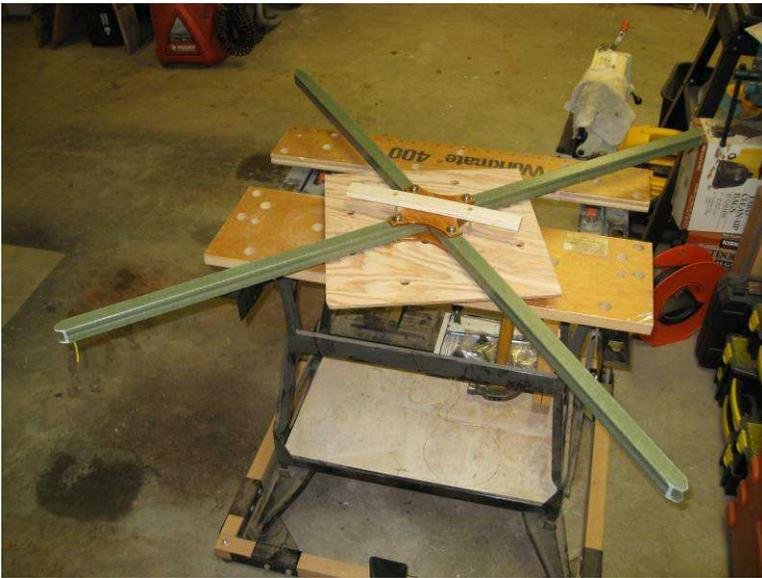
After parts were permanently assembled, the loop frame was clamped to a wood plate with a mandrel on then placed on a shop table for winding. The spool of magnet wire was placed on another mandrel clamped to an adjacent table.
