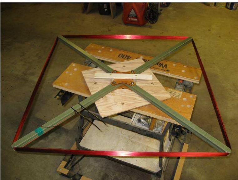
Completed loop antenna with 96 turns and about 1100 ft of wire. 32 turns were later removed as discussed in the measurements section leaving about 720 ft on completed antenna.
