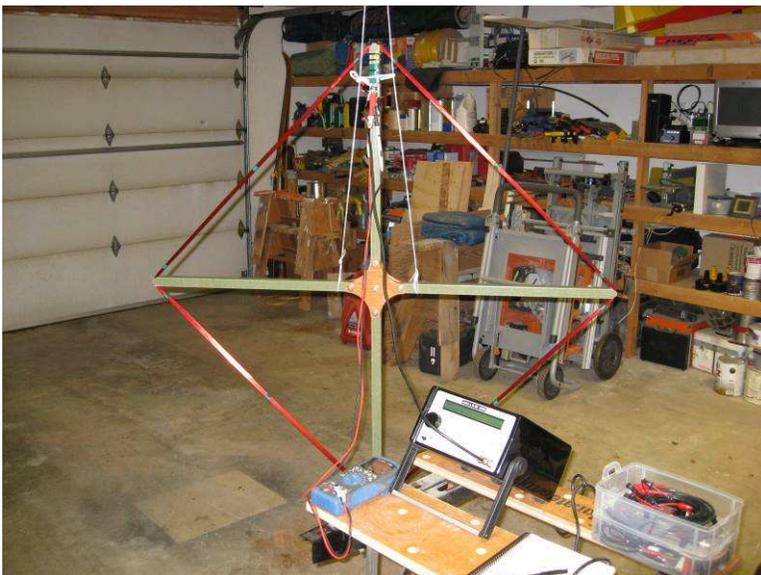
For self-resonant frequency measurements in 2009, a Telulex SG-100A signal generator and Tektronix TDS 2022B oscilloscope was used. The signal generator 50 ohm output was isolated from the loop with 10 kohm and 500 kohm resistors. Measurements were duplicated in 2018 using this setup (but with a different oscilloscope).
