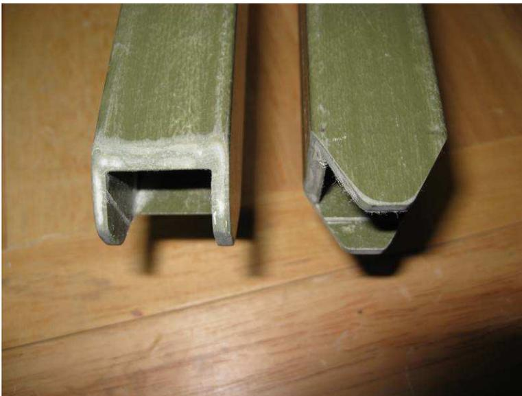
The ends of each brace were cut at 45 angle on the table saw and lightly sanded. The notched ends hold the wire in place.
