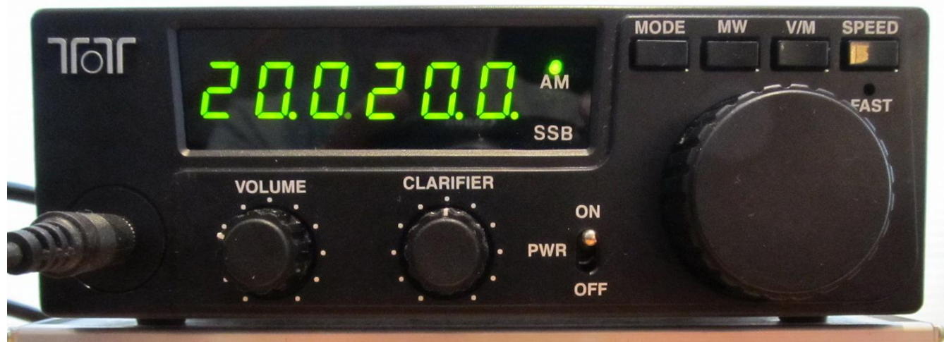
Figure 1 ~ Ten-Tec 1254 receiver in operation. The 1254 tunes in steps of 5 kHz in AM mode or 2.5 kHz in SSB mode (LEDs to the right of the frequency display indicate the mode). The Clarifier control is used for fine tuning. The decimal point on the far-right of the frequency display indicates variable frequency tuning (on) and memory tuning (off). A convenient feature is a Fast tuning mode in which the tuning dial changes the frequency in 0.1 MHz steps. Up to 15 frequencies can be stored in memory using the MW (memory write) function key. The receiver has a built-in speaker, which is muted when an external speaker, headset or soundcard is connected to the speaker jack on the lower-left-front panel.
