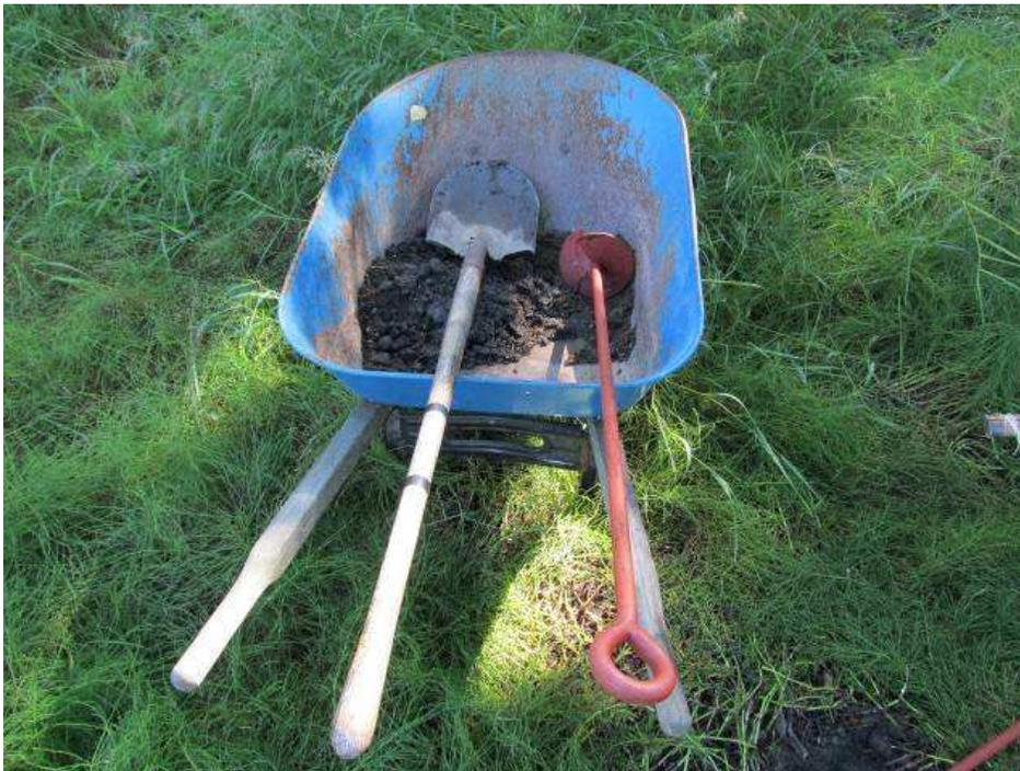
1. To start installation, gather the tools, a shovel and axe handle (not shown), and screw anchors. The screw anchor shown on the right side in the wheel barrow has a 48 in long by 5/8 in diameter shaft with 6 in auger on one end and a single eye on the other.
