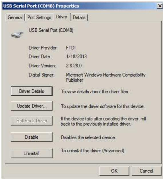
Figure 3.2 ~ Device Driver Properties – Driver tab for a USB-Serial Adapter.
