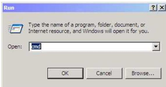
Figure 2.1 ~ Run dialog box and entry to open the **Command Prompt**.
