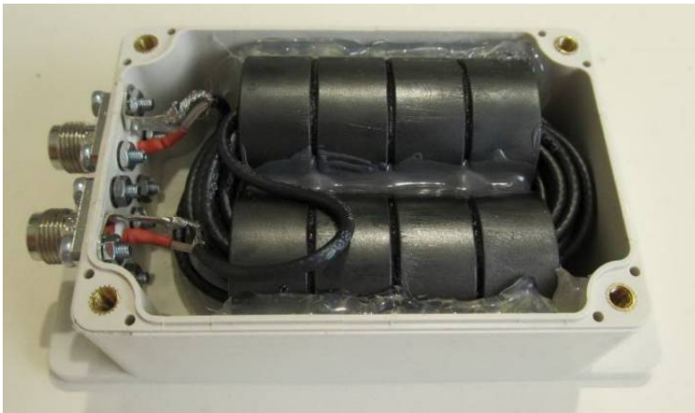
Figure 7 ~ Interior view of the choke with TNC connectors. Hot glue holds the binocular core in place. The coax shield is soldered to a ground lug on each connector flange. ©2020 W. Reeve
