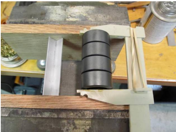
Figure 3 ~ Alignment and clamping of each half of the binocular core. Two 1/2 x 2-3/4 in aluminum angles were clamped laterally in a vice and then the two blocks of four toroid cores each were placed on the angles for alignment. One of the angles is visible at the left-middle. Each block was held together with a non-metallic hobby clamp that uses a rubber band as seen with four toroids at the right-middle. The clamp was left in-place while the glue cured for 24 h. ©2020 W. Reeve
