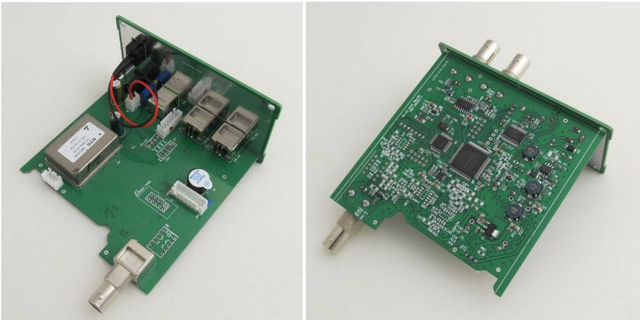
Figure 2 ~ Main printed circuit board top (left) and bottom (right) views, both with the PCB fastened to the rear panel (it is removable). All components on the main PCB except the oven-controlled crystal oscillator, piezoelectric beeper and ribbon connectors are surface mounted devices on the bottom. The oven-controlled crystal oscillator is the rectangular metal box
