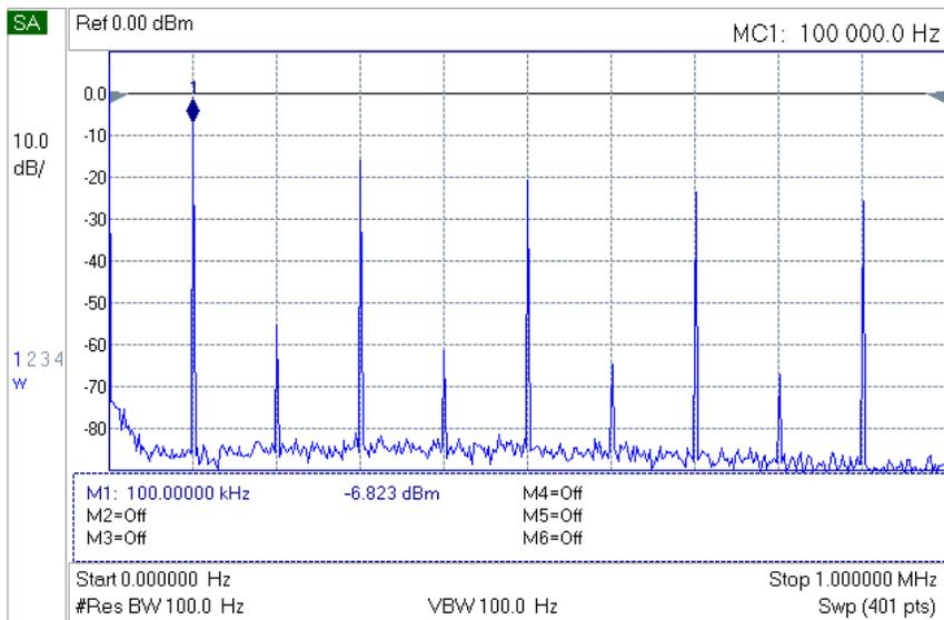
Figure A.4 ~ 100 kHz spectra with 20 dB attenuator between the output and spectrum analyzer. Horizontal sweep is from 0 to 1 MHz.
