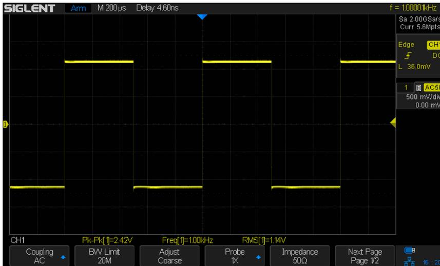
Figure A.1 ~ 1 kHz oscilloscope screenshot. Vertical scale 500 mV/div and horizontal scale 200  $\mu\text{s}/\text{div}$ .
