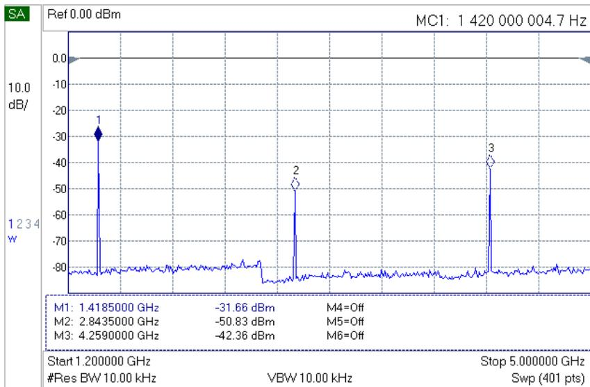
Figure A.11 ~ 1420 MHz spectra with 30 dB attenuator between the output and spectrum analyzer. Horizontal sweep is from 1200 to 5000 MHz.
