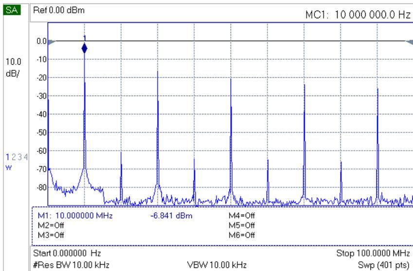
Figure 8 ~ Spectrum analyzer display for the 10 MHz output on channel 1 with the frequency span set to 100 MHz. The spectrum analyzer was connected through a 20 dB attenuator so 20 dB needs to be added to the vertical scale measurements. Horizontal sweep is from 0 to 100 MHz.
