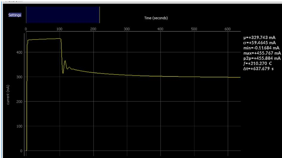
Figure 4 ~ Screenshot from the JouleScope application software showing the WB-SG1 load current (vertical scale in mA) over time (horizontal scale in seconds) for the first 10.5 minutes. The plot starts a few seconds before the signal generator was turned on. The initial warmup period lasts about 2 minutes (left side of plot) and then the current steps down. It subsequently slowly decreases as the OCXO temperature stabilizes.
