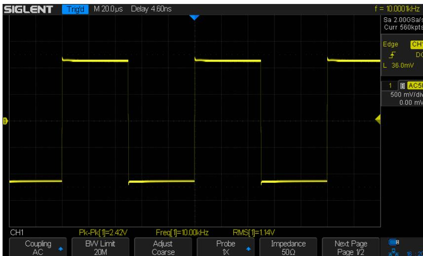
Figure A.2 ~ 10 kHz oscilloscope screenshot. Vertical scale 500 mV/div and horizontal scale 20  $\mu\text{s}/\text{div}$ .
