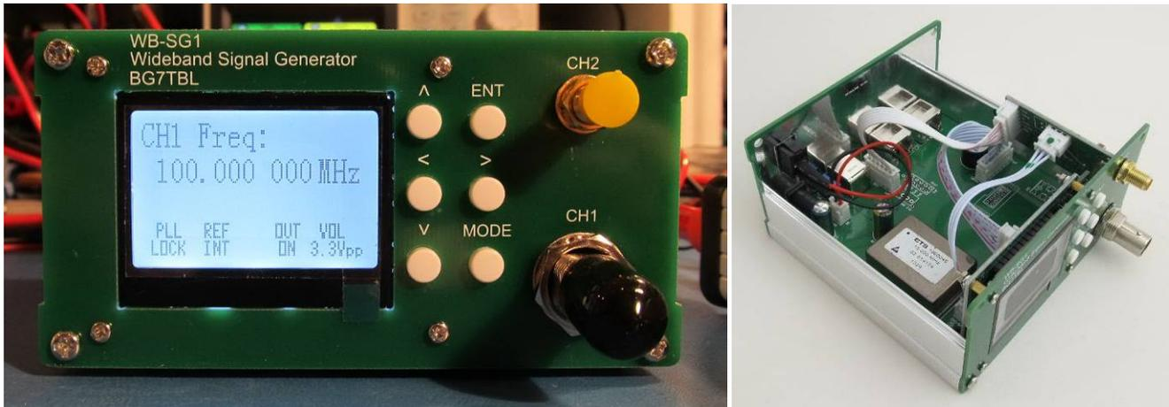
Figure 1 ~ BG7TBL WB-SG1 wideband RF signal generator front view (left) and with top cover removed (right). The dimensions are 106 W x 55 H x 106 L mm (not including connectors) and the weight is 0.35 kg. The connectors for the two output channels, six push-button controls and liquid crystal display are located on the front panel. Images © 2020 W. Reeve
