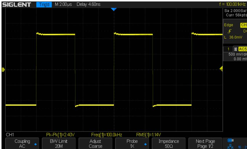
Figure A.3 ~ 100 kHz oscilloscope screenshot. Vertical scale 500 mV/div and horizontal scale 2  $\mu\text{s/div}$ .
