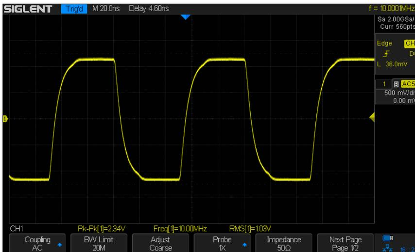
Figure A.7 ~ 10 MHz oscilloscope screenshot. Vertical scale 500 mV/div and horizontal scale 20 ns/div.
