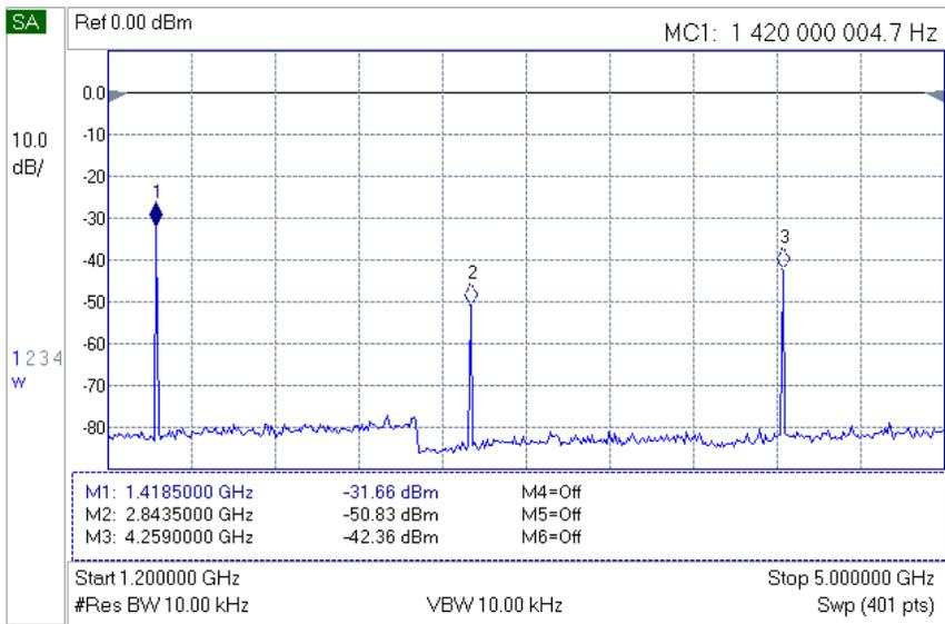
Figure 9 ~ Spectrum analyzer screenshot of showing 1420 MHz fundamental and 2<sup>nd</sup> and 3<sup>rd</sup> harmonics. Add 30.5 dB to the marker levels to account for the external attenuator on the spectrum analyzer input and loss in the connecting coaxial cable. The step in the noise floor just before the 2<sup>nd</sup> harmonic is from the signal generator. The frequency span is from 1200 to 5000 MHz.
