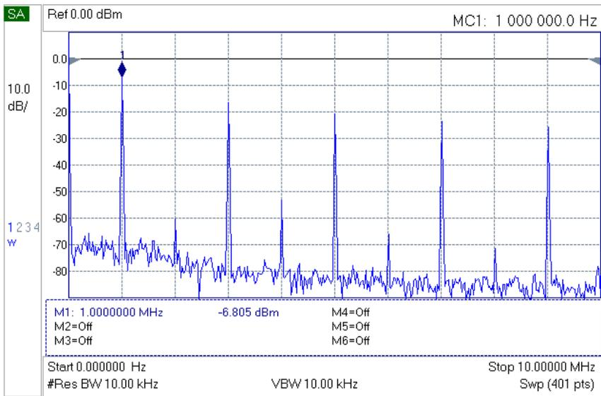
Figure A.6 ~ 1 MHz spectra with 20 dB attenuator between the output and spectrum analyzer. Horizontal sweep is from 0 to 10 MHz.
