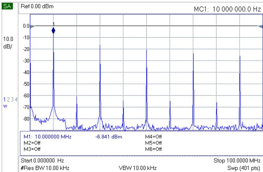
Figure A.8 ~ 10 MHz spectra with 20 dB attenuator between the output and spectrum analyzer. Horizontal sweep is from 0 to 100 MHz.
