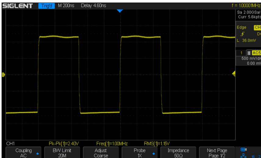
Figure A.5 ~ 1 MHz oscilloscope screenshot. Vertical scale 500 mV/div and horizontal scale 200 ns/div.
