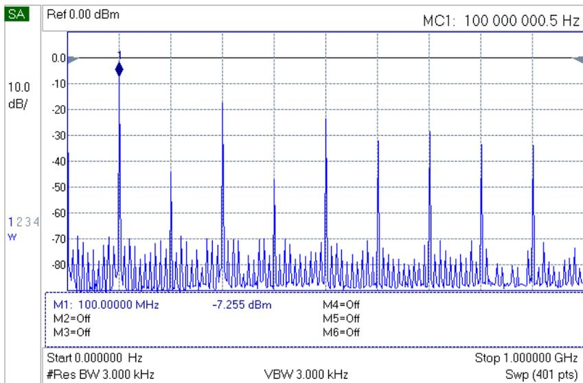
Figure A.10 ~ 100 MHz spectra with 20 dB attenuator between the output and spectrum analyzer. Note the many low-level (approximately -60 dBc) spurious signals compared to lower frequencies.
