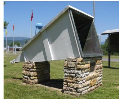
at Harvard in the USA, who found the predicted 21 cm wavelength hydrogen line in 1951. They used a hand-built plywood and copper 1,420 MHz horn antenna (their original horn antenna is on display at NRAO Green Bank West Virginia, photo above right). As a result of this discovery and its later exploitation, radio astronomers were able to build up a more complete idea of what the whole galaxy is like and to confirm its shape as thought to exist through optical astronomy.
