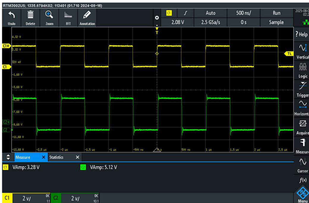
Figure 2 ~ Input (yellow) and output (green) voltage waveforms for the clock buffer IC8. The input waveform is from the LBE-1420 and its amplitude is 3.28 V; the buffer input waveform and voltage from the Mini-GPS is identical. The output voltage from the buffer is TTL level at 5.12 V.
