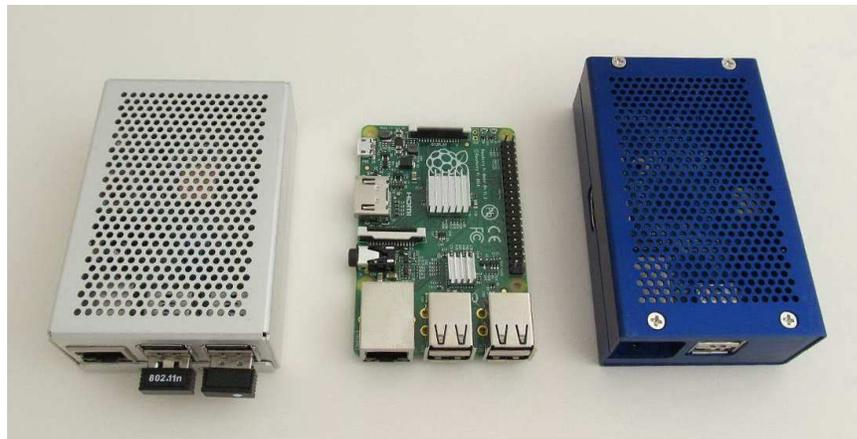
Figure 2 ~ Raspberry Pi model B and B+ hardware. The model B+ is shown in an aluminum enclosure with USB WLAN and BlueTooth dongles (left) and with no enclosure (middle). The model B (right) also is in an aluminum enclosure. The interfaces vary slightly between the model B and B+ but Callisto-Pi works on both models. Enclosure dimensions are approximately 100 x 65 x 25 mm. (Image © 2014 W. Reeve)
