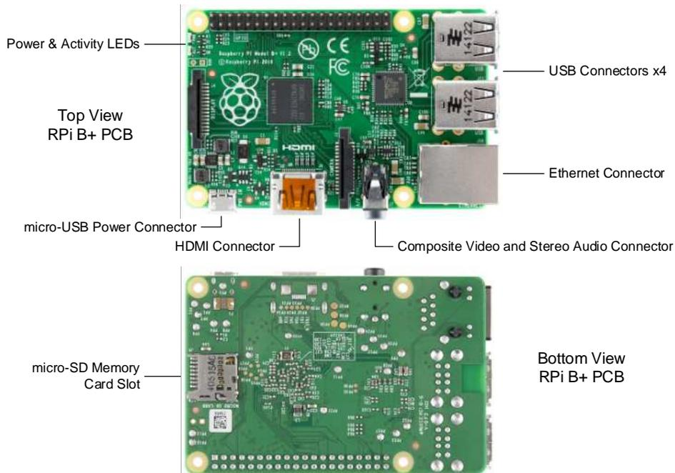
**Memory card:** Install the memory card. The RPi model B uses a full-size memory card carrier in an ordinary push-to-insert/pull-to-release slot connector. The model B+ uses a micro-SD memory card in a push-to-insert/push-to-release slot connector.
