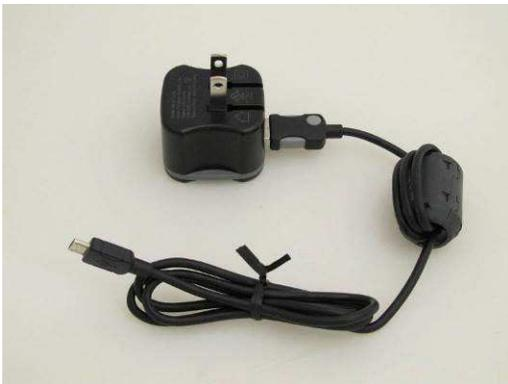
AC wall power adapter with North American ac input plug. One or more clamshell ferrite beads on the dc power lead may help reduce radio frequency interference from the switch-mode power supply. This image shows one bead on the right with three windings of the power lead. The Raspberry Pi uses a micro-USB connector for power. (Image © 2014 W. Reeve)
