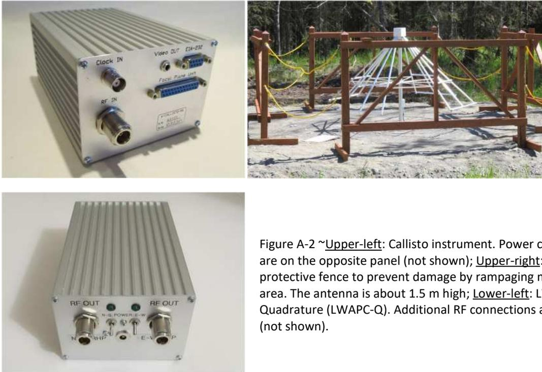
Figure A-2 ~Upper-left: Callisto instrument. Power connections and control are on the opposite panel (not shown); Upper-right: LWA Antenna with a protective fence to prevent damage by rampaging moose that frequent the area. The antenna is about 1.5 m high; Lower-left: LWA Power Coupler – Quadrature (LWAPC-Q). Additional RF connections are on the opposite panel (not shown).
