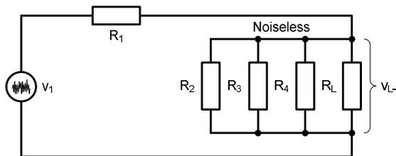
Fig. 2-6 – Equivalent voltage divider circuit.  $V_{L-1}$  is the noise voltage across the load resistor due to  $R_1$
