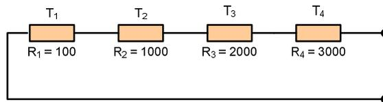
Fig. 2-8 – Example series resistor combination
