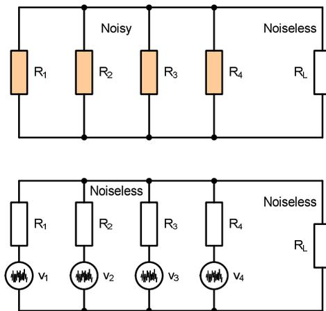
Fig. 2-5 ~ Combining noise sources. The noisy resistors (upper) are replaced by their equivalent noise models (lower).
