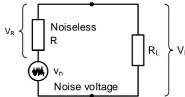
Fig. 2-4 ~ Noisy resistor model under load
