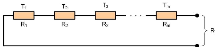
Fig. 2-7 – Series resistors
