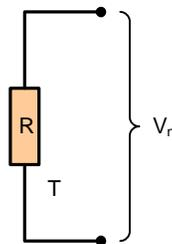
Fig. 2-1 ~ Resistor with resistance  $R$  at temperature  $T$  produces an open-circuit noise voltage  $V_n$ .
