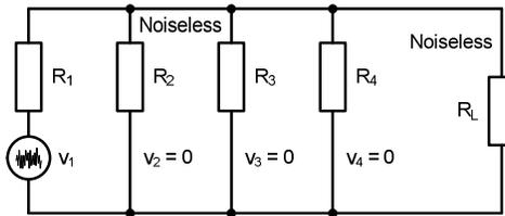
Fig. 2-9 – Example noise resistor network with  $v_2$  through  $v_4$  shorted out
